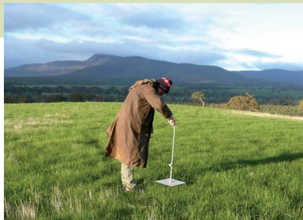
Measuring pasture with a rising plate meter
