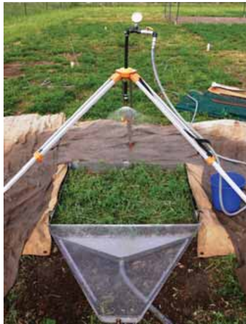
Fig. 2. Portable rainfall simulator delivering a rain storm of 105 mm/h for 30 minutes on a lucerne + digit grass pasture mixture.
